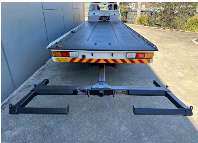
Under-body wheel lift and tow bar assembly, stowed at the rear of the unit
