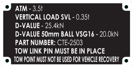
Tow bar rating plate — ATM, vertical load and D-value
