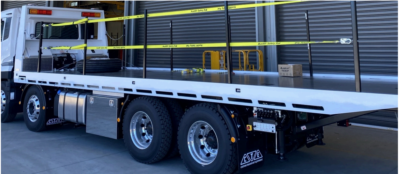
Fall protection installed along the tray
