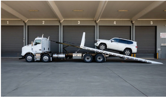
Winching the load up the tray at a low angle
