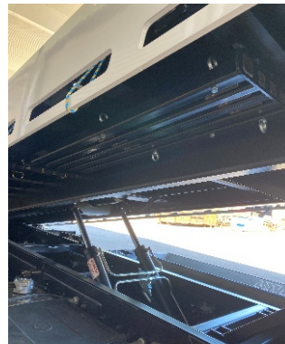
Pole storage space under the tray
