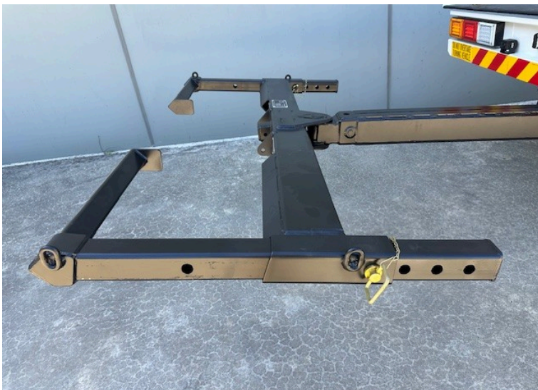
Tow bar / wheel lift assembly, fully retracted with mechanical pins fitted
