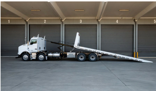
Tray fully slid back, tilted and extended to the ground
