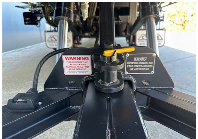
Safety pin at the wheel lift lock — must be installed at all times while in transit
